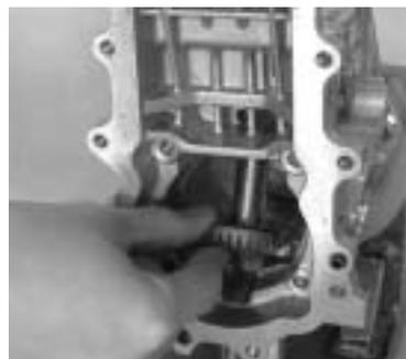
Remove the transmission shaft CMP.
