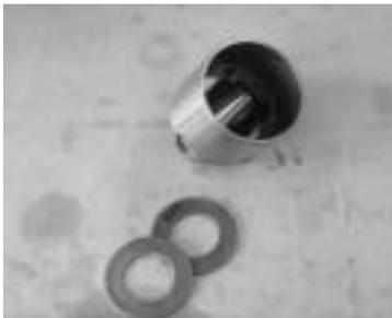
Tappet disassembled and FIC adjust shim.
