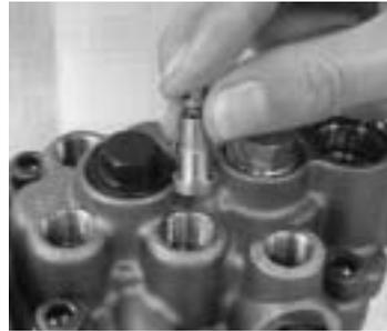
Install the delivery valve CMP.
