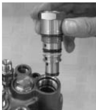
Install the holder with new O-ring, (timer).
