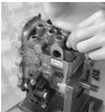
Install the hydraulic head CMP.
