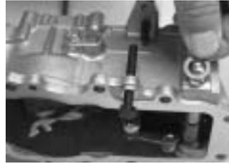
Install the shim to the shaft, (control lever).
