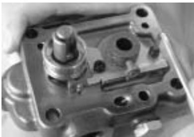
Remove the rack guide fastening bolt.
