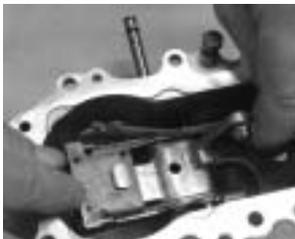
Pierce the governor lever CMP and shim through the governor lever shaft and assemble.
