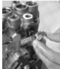
Remove the plug, (accumulator).
