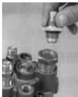
Install the thermo-element with new O-ring.
