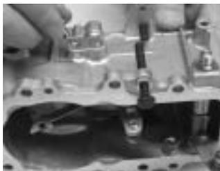
Fit the governor lever shaft with the removal stop, (governor lever shaft) and fasten the removal stop bolt.
