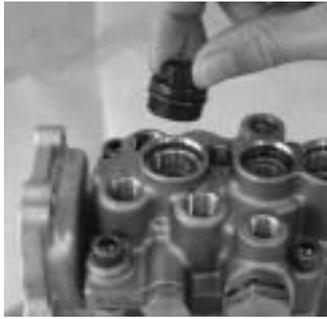
Install the plug, (distribution shaft).
