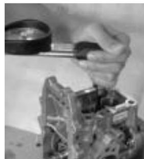
Fasten the removal stop, (transmission shaft).
