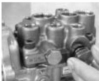
Install the plug with new seal washer, (accumulator).
