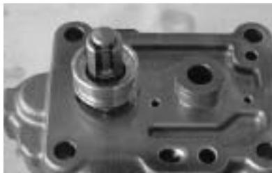
Install the control sleeve and spring retainer.
