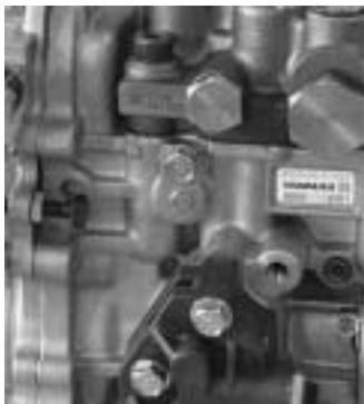
Remove the link lifter fix bolt.
