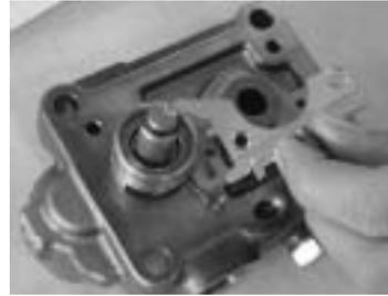
Remove the spring retainer.
