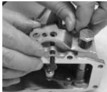
Pierce the spring, (control lever) through the lock nut, (control lever) and fasten it to the thread of the shaft, (control lever).
