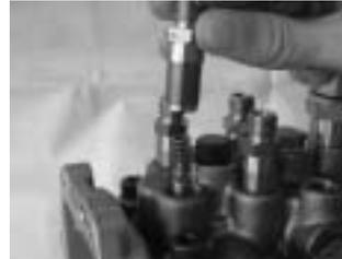
Remove the delivery valve and gasket.
