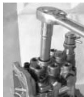
Remove the delivery valve and gasket.
