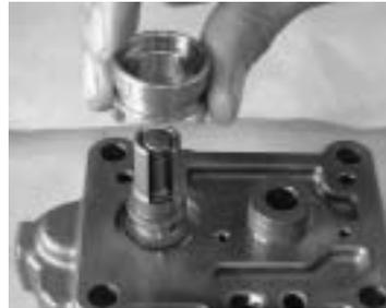
Remove the control sleeve.
