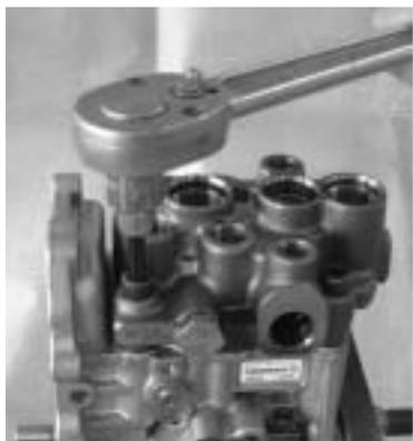
Remove the hydraulic head CMP fixing bolt.
