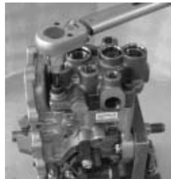
Install the hydraulic head CMP fastening bolt.
