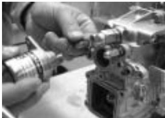
Install the new U-ring to the stop solenoid and assemble them to the governor case.
