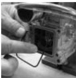
Install a new packing, (governor case cover) to the case.
