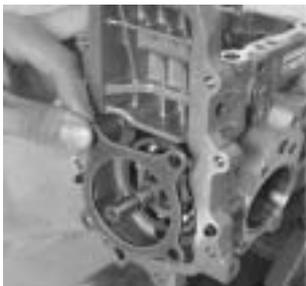
Remove the retainer, (bearing).
