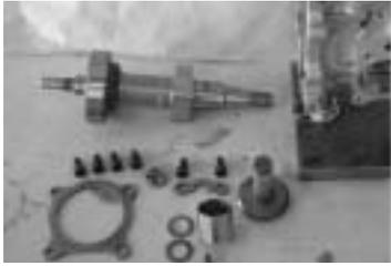
Remove the transmission shaft CMP.
